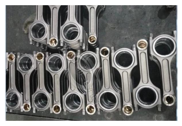
3). Heat treated to HRC 34-38 and polished and finally shot peened for high fatigue strength.
