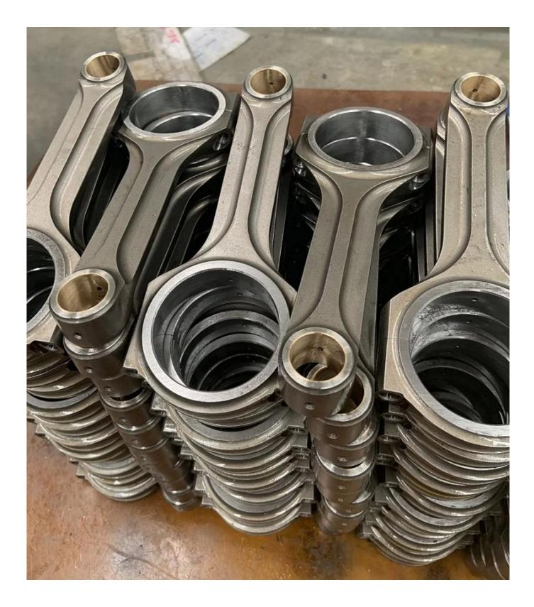
Those Forged 4340 Steel Connecting Rods for 4G63T Engines are ready for cleanning, inspecting and packing.
