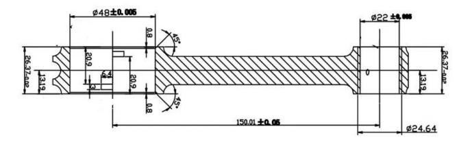
This is our forged 4340 steel connecting rods main size with tolearance and bearing tag dimension.
