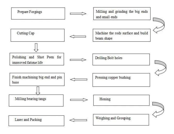
Hurricane produces 4340 forged connecting rods for a wide range of applications, include I Beam, X beam and H beam shapes ,
