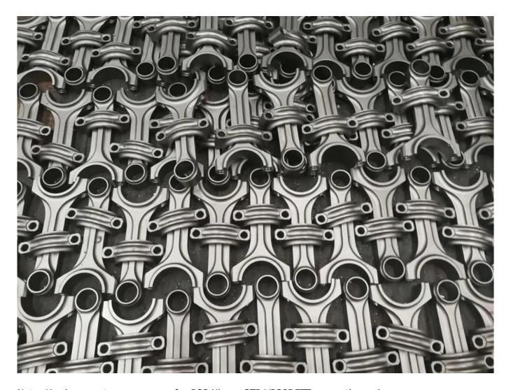
Note: Hurricane cut cap progress for R35 Nissan GTR VR38DETT connecting rods
