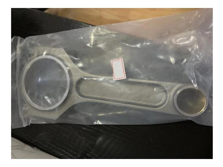
Ford Modular 5.4L 5.8L Connecting Rods are fitted with hurricane 7/16 bolts and silicone bronze wrist pin bushes to ensure reliability. each set are balance weighted in +/-1 gram.
