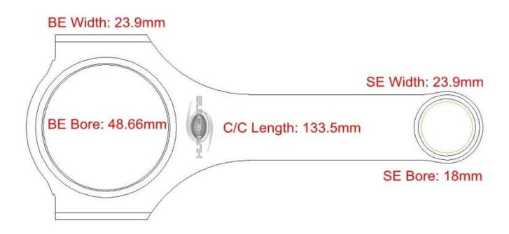
Citroen / Peugeot 106 GTi / S16 1.6L TU5J4 133.5mm Connecting Rod H-Beam are manufactured from 4340 high tensile steel and are designed for high performance and extreme durability. They are shot peened to relieve stress from the material and multi-stage heat treated to increase rigidity. The tight tolerances in the production process, ensure a perfect fitment while optimizing the oil clearances. Bend and twist is tightly controlled.
