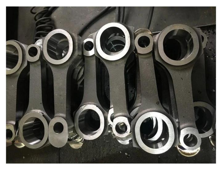
This is a progress of drill big and small end bore, which acts as a reliable locator in all process. Hurricane BMW M60 143mm forged Connecting Rods are designed for the applications where rod strength is the number one concern rated in excess of 1000+ horsepower(HP) per set. they are fits for BMW E38, E39 - 4.0 4.4 V8 engines.
