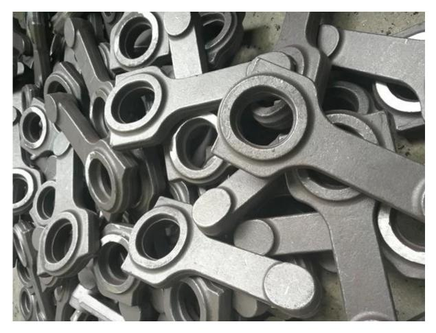
Every rod is shot peening to stress relieve the metal. x-rays, measure, and Magna-fluxes each rod to ensure quality. Every rod is multi-stage heat treated. And if necessary, Hurricane 7/16 bolt can be installed and provided.
