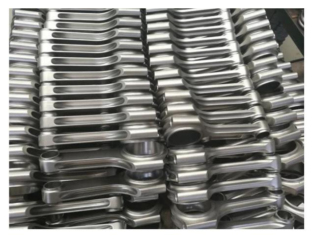
Silicon bronze bushings are inserted for a floating piston pin.
