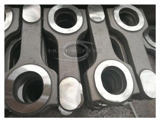
They are heat treated to HRC 34-38 , then **polished and shot peened** to provide more fatigue strength. All these rods small ends are bushed for a fully floating pin and packed in balanced sets well +/-1 gram, and are available with 7/16" ARP 2000 bolts .
