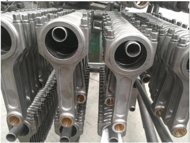
They could come standard with 190,000 psi rated ARP 8740 and 230,000 psi rated ARP 2000 rod bolts, or 265,000 psi rated ARP L-19 bolts as upgrades. Instructions and rod bolt lubrication are included.
