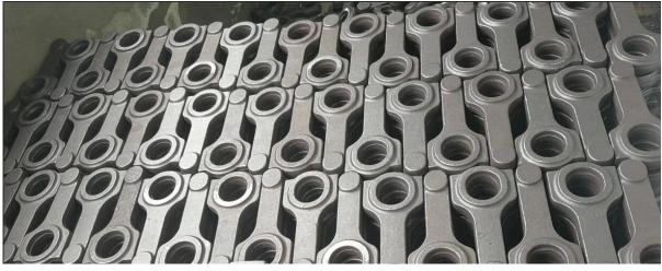
Then, Machining them on CNC machine, shot peening, blasting hone bore
