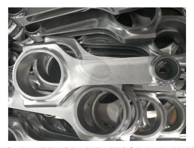
Per rod comes with high quality bronzed bushing suitable for floating piston pin, and dowels located t he rod cap to achieve accurate assemble. What's more, all the small ends and big ends are honed b y SUNNEN honing machine to meet high tolerance standard, so they are a good choice for your high performance engines.
