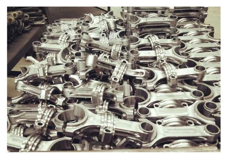
Hurricane have H beam, X beam and I beam design for Buick Series II L67 V6 connecting rods.
