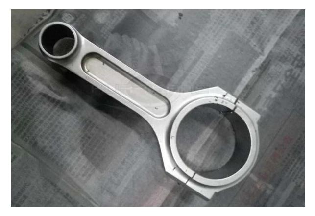
What's more , per 7.100 " connecting rods are inserted with highly durable bronze bushings for floating piston pin, high quality dowels installed on each rod for perfect fit and accurate re-assembling .
