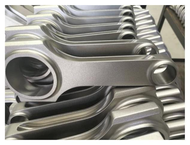
Fully CNC machining for superior tolerances
