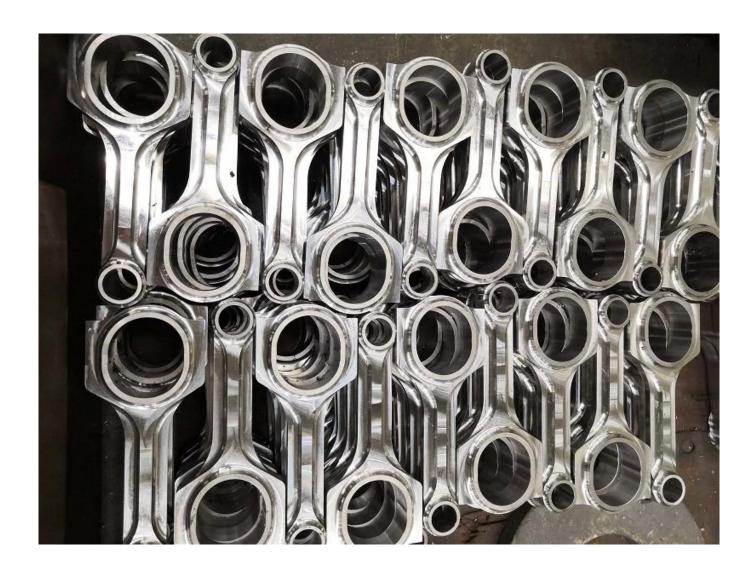
Note: This is the picture after milled X beam bmw connecting rods progress. for more production pro gress, please check our news page: <u>Hurricane High Performance connecting rods - Process of machining rods</u>
