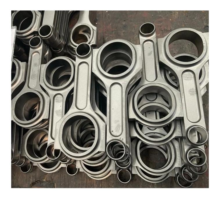
Note: BMW E46 M3 S54 139mm I beam forged steel connecting rods are ready for shot peenning. You can check more details about this progress at News page: <u>Connecting rods Shot Peening and Mirco-Polishing, Special A-level appearance</u>
