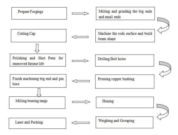
Hurricane connecting rods machined for high performance racing applications , all the rods finish with high technical standard to meet high quality needs . We only show some production process in here, if you are interested in more details , please feel free **contact** us . And welcome to search "Hurricane connecting rods video" on google to view more production videos.
