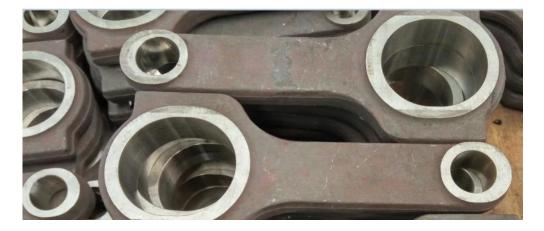
2.Manufactured as <u>**I-beam shape**</u> to provide better combination of light weight and strength, each rod heat treated to HRC 34-38 and then shot peened for a higher fatigue strength , packged with 8pcs/set , Optimal balancing for weight matched  $\pm 1$ gram per set .
