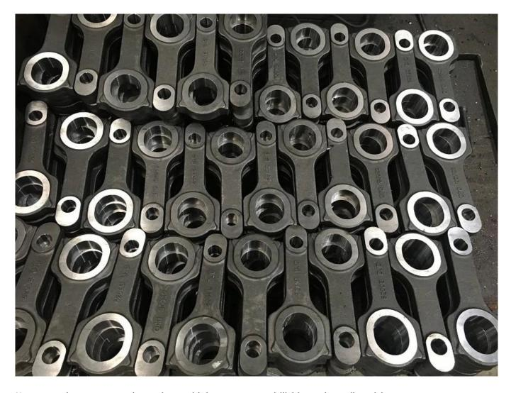
Note: mazda mzr connecting rods machining progress: drill big and small end bore.
