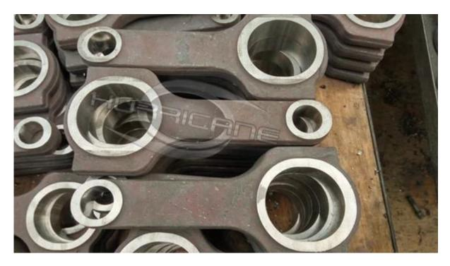
Per rods forged and 100% finished by advance CNC machine at Hurricane CNC center, they are perfectly match Nissan CA15 performance engines. Special dowelled cap for Precision Alignment and sized to tight specifications, shot peeds to relieve stress fully.
