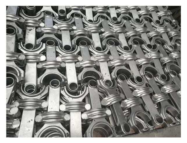
Note:separate cap form connecting rod
