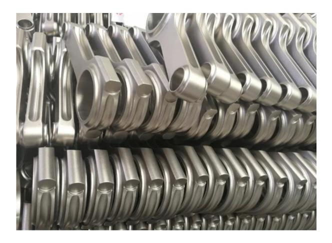
Perfect for Small Block engines and Big Block engines producing up to a valid horsepower. This set of rods makes use of a press-fit to retain the wrist pins.
