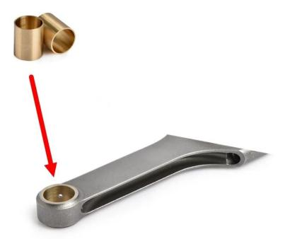
100% X-rayed, sonic tested, magnafluxed and shot peened for improved fatigue life.
