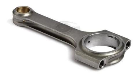
Hurricane connecting rod for Honda B16 are Burried and polished, those processes remove burrs and make surface smooth. also shot blasted, this process means Small ball hit surface and make them on surface, increase rods strength. We also use Sunnen Honing Machine to Hone forged honda rods big and small ends, make all to use sizes and save you time on machine shop. If you want to know more of
