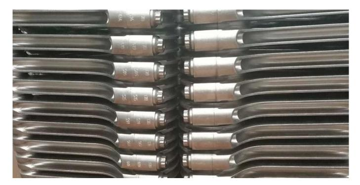
Note: The side of shoulder is also used for permanent identification marks, used specifically for re-uniting the rod and its cap after the parting tool makes it cut. You can check more progresses detailed information at: <u>Hurricane High Performance connecting rods - Process of machining rods</u> Or check our opreations at Youtube Viedo: <u>How it's made: Connecting rod</u>
