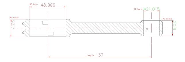
H Beam Connecting Rods for Honda / Acura B18A B18B B20 Engines Features
