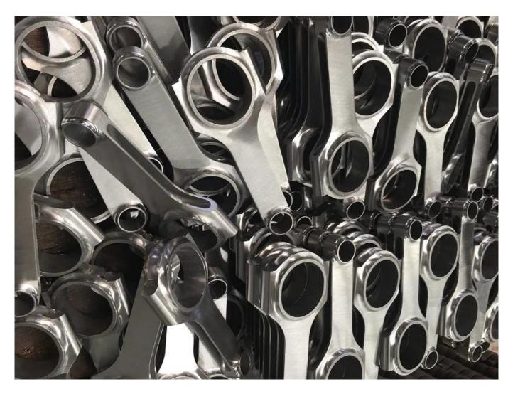
Note: This is one of our crucial operations in the making of a competition connecting rod.: Micro Polishing. it will enhance rods durability while leaving a great-looking finish. You can check this News Page to get more detailed information: <u>Connecting rods Shot Peening and Mirco-Polishing, Special A-level appearance</u>
