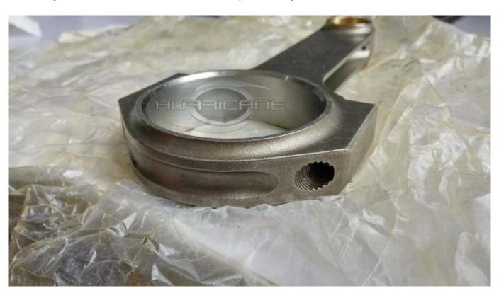
The Big end bore is machined on CNC advance manchiny and honned on Sunnen Honing Machine. So the surface is very smooth and it`s precision is within 0.01mm after honing. Much more Hurricane Air cooled connecting rods bearing tag can fits oem spec bearings.
