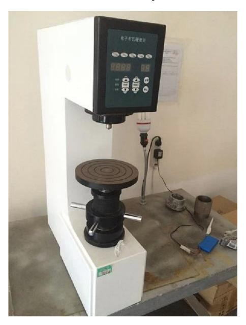
Note: this is our Hardness Test Machine, Hurricane connecting rods hardness 34-38 HRC.
