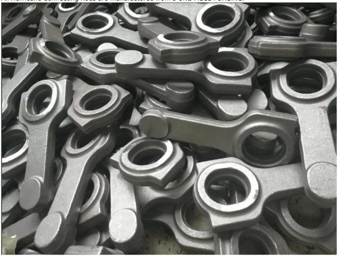
The forging process forces the grain into the shape of a connecting rod, resulting in a superior fatigue life.
