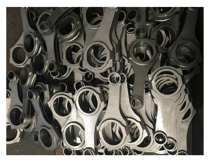
Presenting a new Pro H profile connecting rod for the Subaru BRZ / Scion FR-S FA 20 engine. Micro Polishing enhance rods durability while leaving a great-looking finish and Shot Penning the surface of the conrods can relieve stress, improved fatigue life. for more information, please check our news page: <u>Connecting rods Shot Peening and Mirco-Polishing, Special A-level appearance</u>
