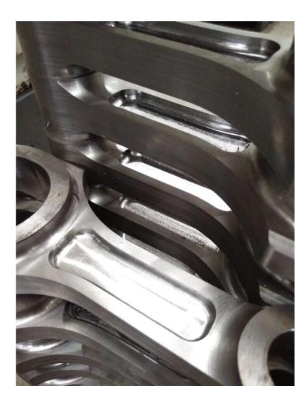
The duramax diesel connecting rods strong tapered I beam configuration can handle extreme engine loads. The tapered beam allows for some weight saving on the reciprocation end and gives increased clearance for fully boxed pistons.
