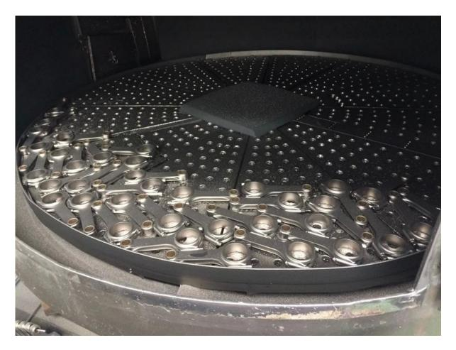
Note: As a quality rods manufacturer in racing industries, all the Hurricane connecting rods are shot peened fully with steel balls at factory to improve fatigue life to enhance strength , and also help to make the rods be more beautiful and smooth .
