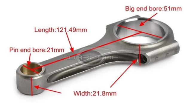
**Hurricane Speed and Performance** H-Beam connecting rods - Nissan RB26/RB25 are manufactured from **4340 steel forgings**, then They are fully machined, heat treated, stress relieved, shot peened, and magnafluxed, **all process of machining rods** post on website. Final all connecting rods Weight matched to +/- 1.5 grams. Perfectly round big and small ends. Bend and twist is tightly controlled. Cap fasteners are **3/8" ARP 2000 for the H-Beam and 3/8" ARP Custom Age 625+ for the H-Plus**.
