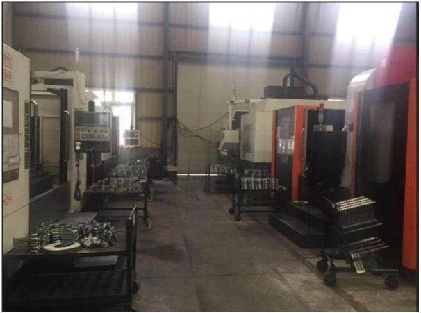
These machine mill, grind and drill on the connecting rod. Most factories used to machine with worker, which was a time consuming process. In order to reduce the time and improve rods quality, at present all rods machined with full CNC MACHINE.
