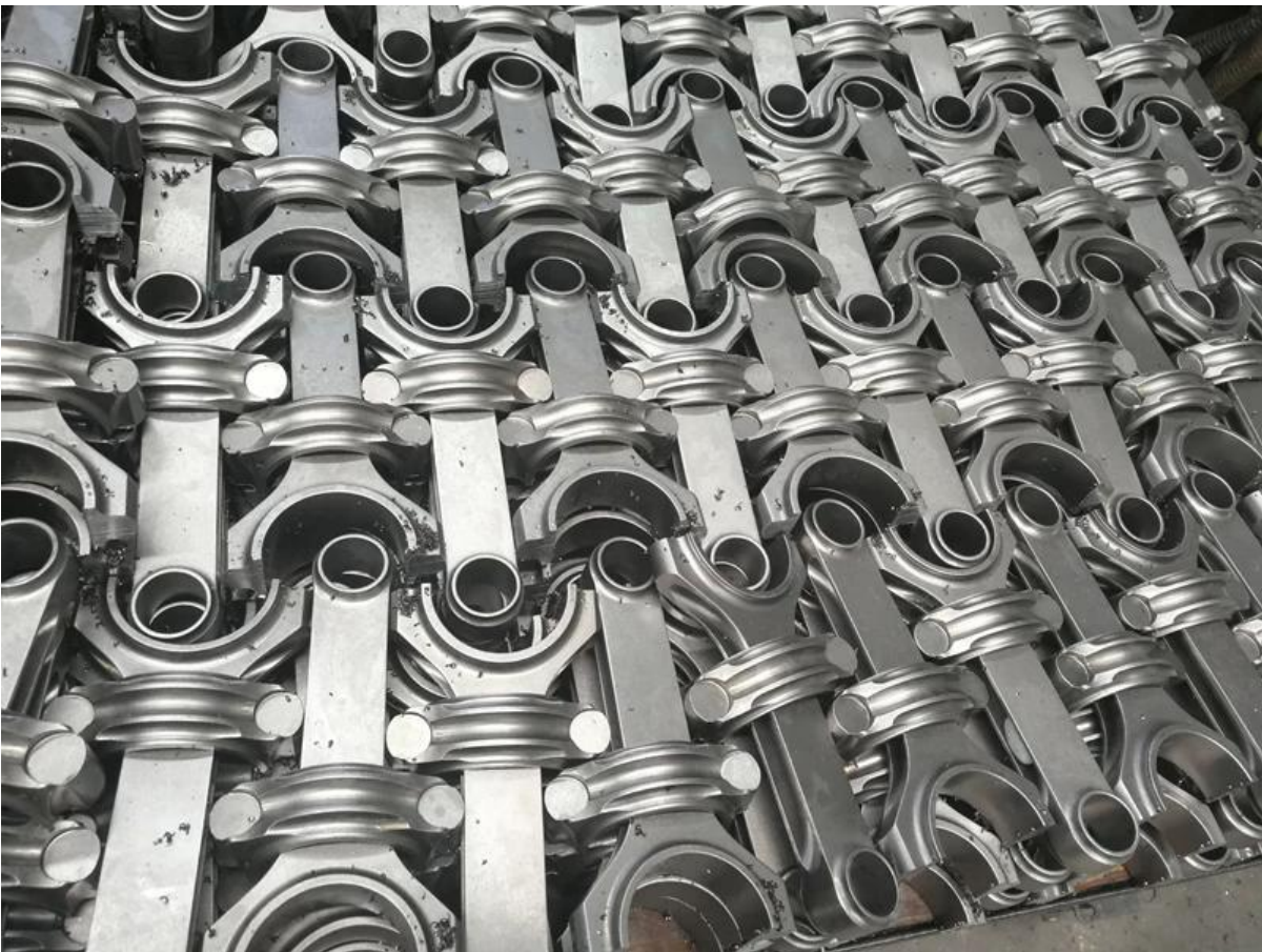
Note: Cut cap, make cap leave from the whole rods
