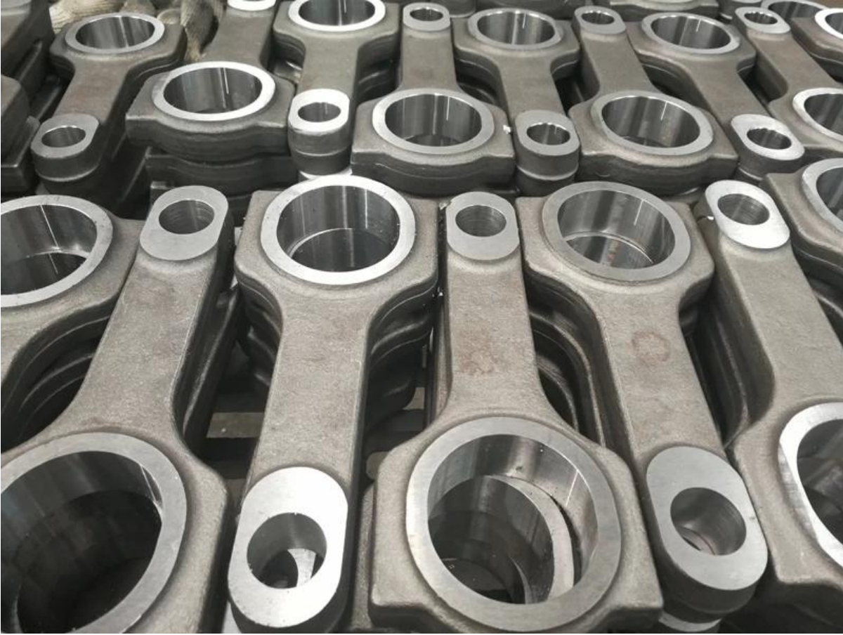
Note: drill big end bore and small end bore
