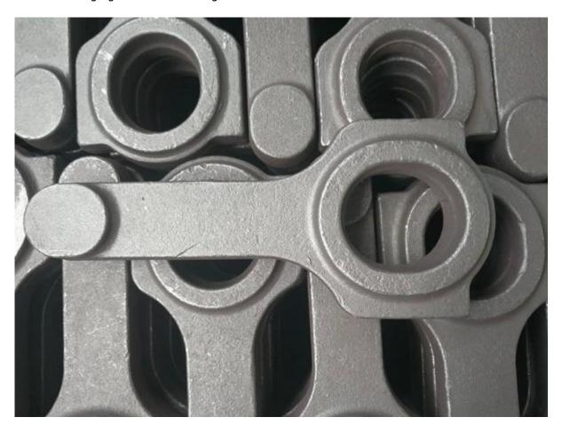
The forged blank should be quenched and tempered with HRC34-38 hardness.
