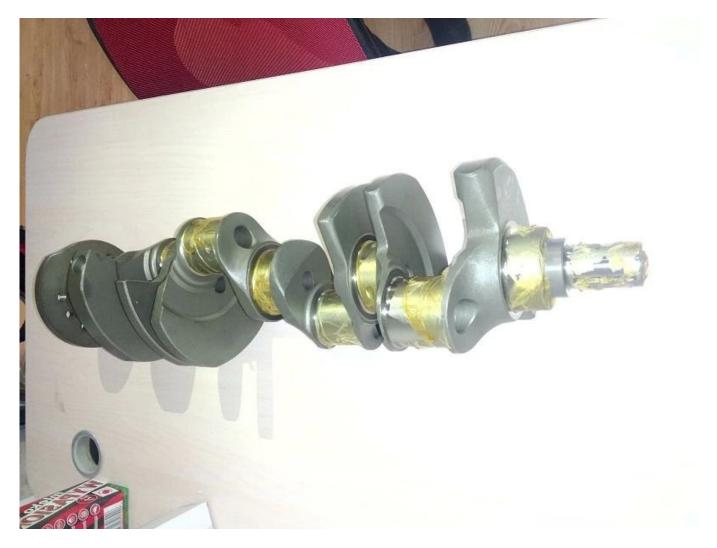
Here is our finished 4340 forged steel crankshaft for Chevy 350 sbc engine. except 3.250" stroke, we can also offer
